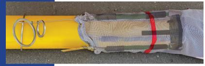
After placing the safety collar around the pipe, the pipe slides into the mesh down to the stop plate shock system.
