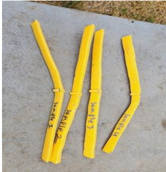
Figure 5. Examples of PA12 pipe specimens which exhibited high-quality fusion.
