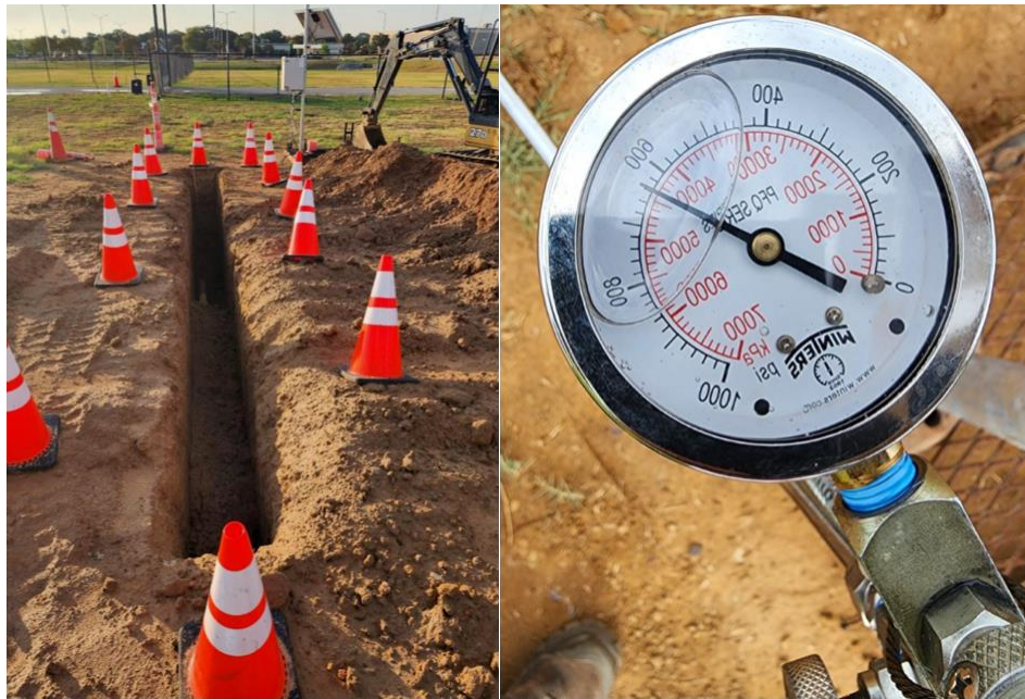
Figure 7. Test setup for sustained pressure testing completed by CoServ.
